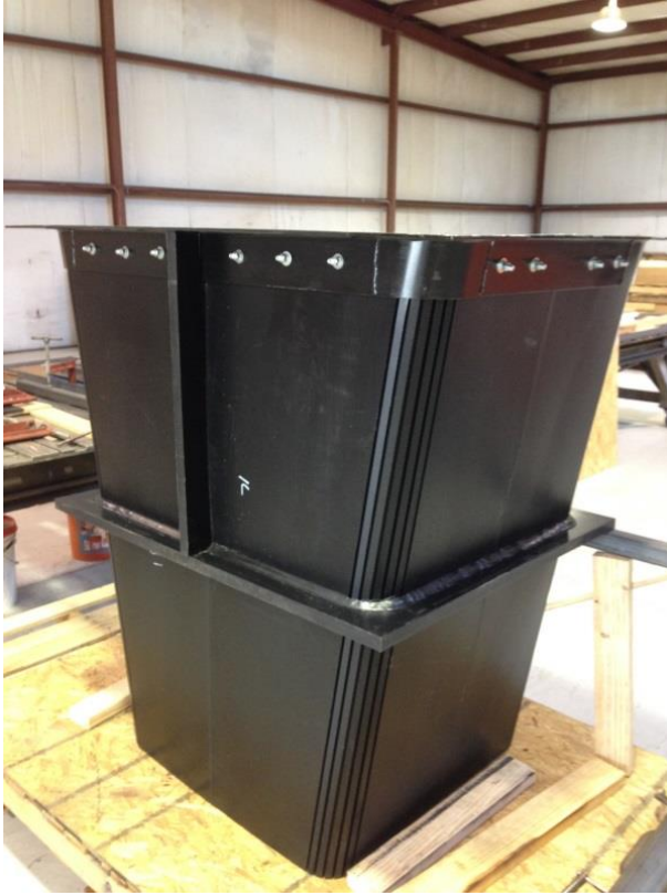
FGD discharge chute fabricated from TIVAR 88-2 ESD with upper steel mounting flange.
