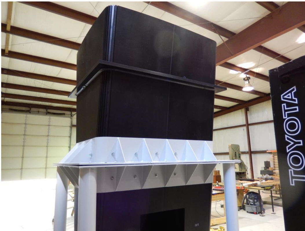
FGD transfer chute hopper fabricated from TIVAR 88-2 ESD material with steel support frame.
