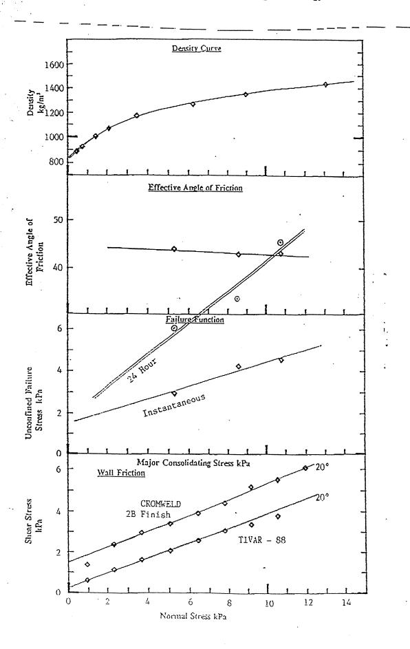
General flow test results from the gypsum tested (6.03% moisture before testing, 5.03% afterwards)
