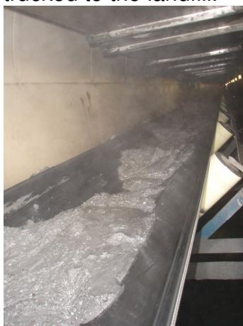
Figure 1 – Scrubber sludge after it has been mixed with fly ash and lime
