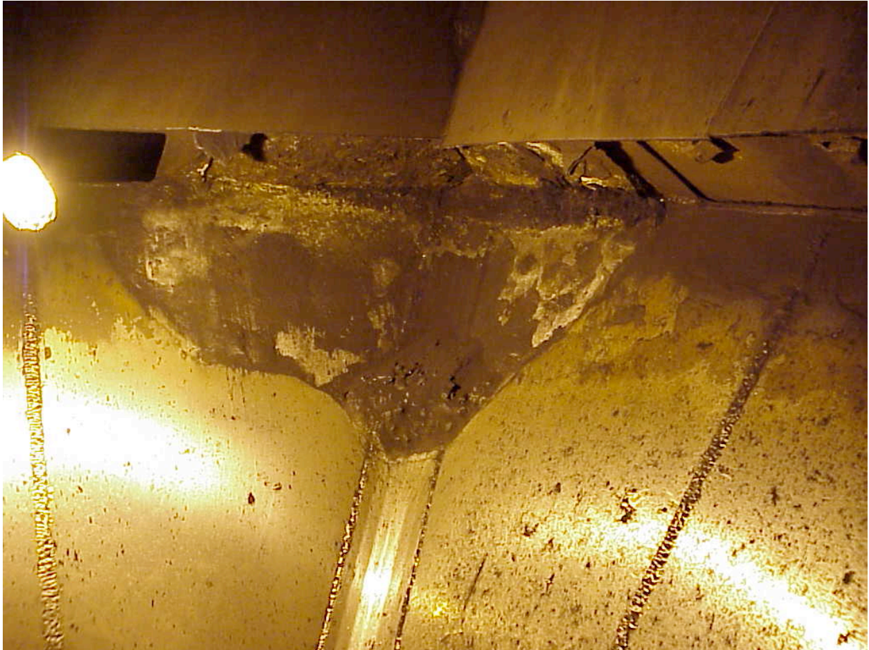
Figure 5: Buildup of coal in the corners of the discharge hopper and surface corrosion and pitting on stainless steel liners.
