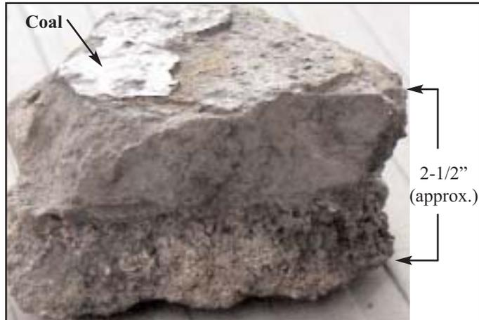
**Figure 1.** Typical gunite coating portion
