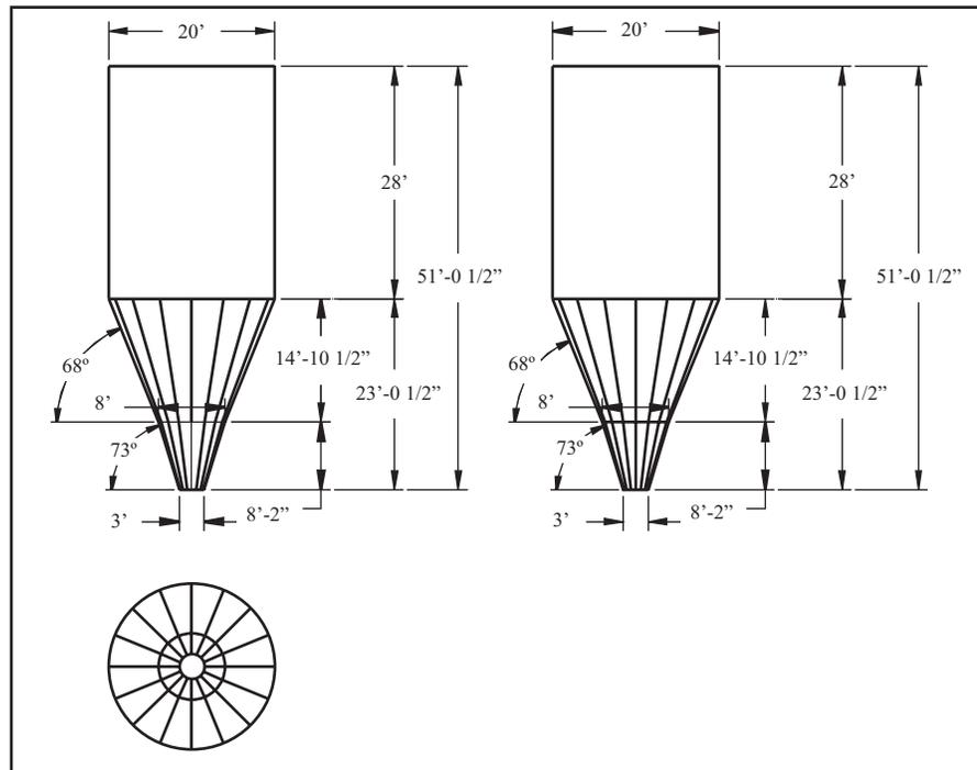
**Figure 5.** Unit 5 bunker modification with symmetric two-stage conical hopper.
