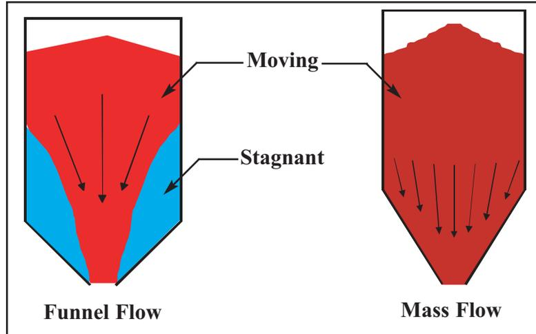
Figure C. Funnel flow and mass flow
