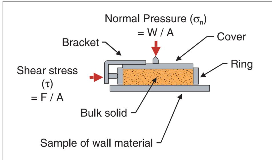
**Figure E.** Wall friction test
