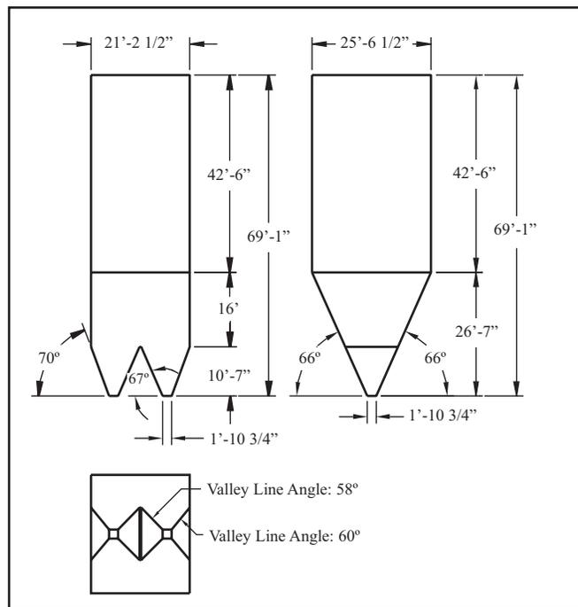
**Figure 6.** Unit 8 bunker dimensional layout
