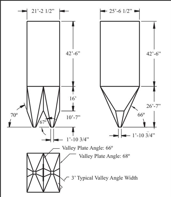
**Figure 8.** Dimensional layout for Unit 8 bunker valley angle clean out plate modification
