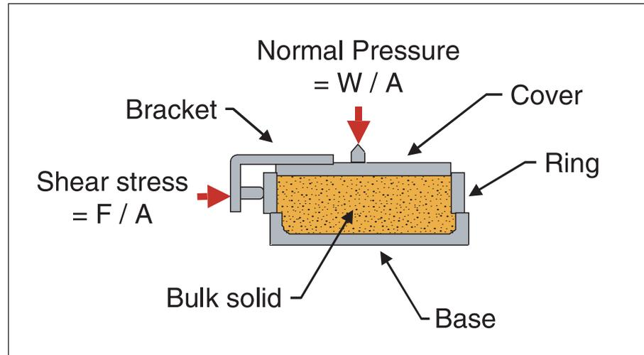
**Figure F.** Shear test
