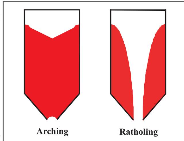
**Figure A.** No-flow problems – arching and ratholing
