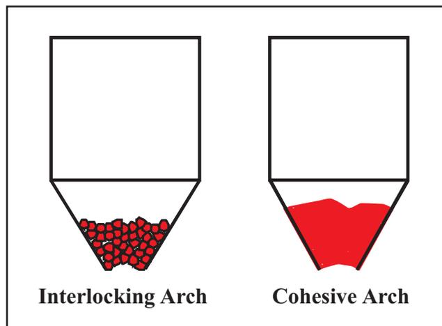
**Figure B.** Arching in a silo – interlocking or cohesive
