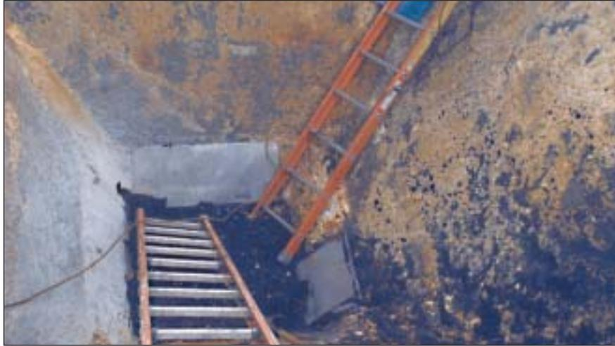
**Figure 8. Kammer reclaim hopper - before TIVAR® 88 installation**
